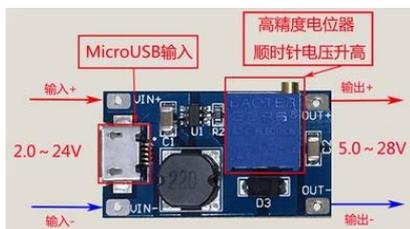
Gambar 3. Modul step up converter MT3608
